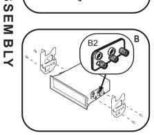
2 Mount the factory brackets to the shaded bosses (Fig. B2) with(4) #8 x 1/4" Phillips Pan Head Screws supplied and mount the entire assembly to the sub-dash. See figure B
