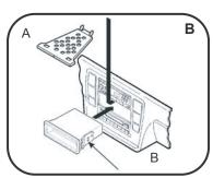
2 Pull out on the plastic tray separating the dash cavity and remove the tray ("A"). Position the Pocket so each Bracket is configured with (2) screws on the top and (1) screw on bottom ("B"). Slide the pocket into the dash opening until the side clips engage.
