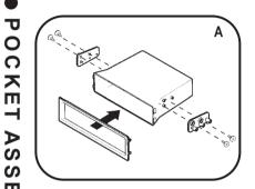
1 Snap Pocket Trimplate MIT onto the front of the Pocket. Locate one of the Left Brackets and mount it to the "L" side of the Pocket with (2) #6 x 1/4" Phillips Flat Head Screws. Next locate one of the Right Brackets and mount it to the "R" side of the Pocket with (2) #6 x 1/4" Phillips Flat Head Screws.
