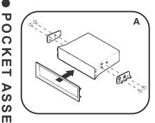
Snap Pocket Trimplate VW (labeled TP-9008) onto the front of the Pocket. Locate the X-5599L bracket and mount it to the "L" side of the Pocket with (3) #6 x 1/4" Phillips Flat Head Screws. Next locate the X-5599R bracket and mount it to the "R" side of the Pocket with (3) #6 x 1/4" Phillips Flat Head Screws .
