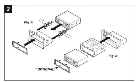
**ISO HEAD UNITS:** Snap the **Trimplate** into the **Radio Housing.** Attach the **ISO Brackets** to the inner lip of the Housing. Slide the head unit into the radio opening, align the holes in the head unit with the holes in the ISO Brackets and mount the unit to the brackets with the screws supplied with the unit. (see Fig.A).
