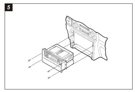
Re-connect the battery terminal and test the unit for proper operationt. Mount the head unit/kit assembly to the sub-dash with (4) Phillips screws previously removed in step #1.
