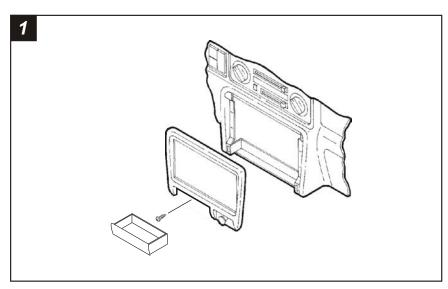
Disconnect the negative battery terminal to prevent an accidental short circuit. Remove the ashtray and (1) Phillips screw exposed in the ashtray cavity. Remove (4) Phillips screws securing the factory head unit and disconnect the wiring.
