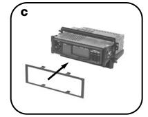
NOTE: To remove the mounted head unit. unclip and remove the ISO Trimplate. Using a small flat-blade screwdriver, disengage the side clips securing the ISO Snap In Brackets to the housing pocket assembly.
