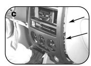
Remove (4) phillips screws to remove radio.
