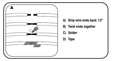
1 Locate the factory wiring harness in the dash. Metra recommends using the proper mating adapter and making connections as shown. (Isolate and individually tape off the ends of any unused wires to prevent electrical short circuit.)
