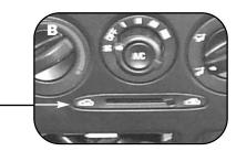
Unsnap and remove radio / climate control bezel.
