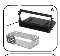
1 Slide the DIN cage into the Radio **Housing** and secure by bending the metal locking tabs down.
