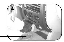
On 2002 models, remove knob from fresh air/recirculate control.
