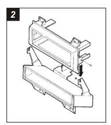
Remove the pocket from the factory head unit and slide the side tabs on the *Radio Housing* between the mounting tabs on the pocket.
