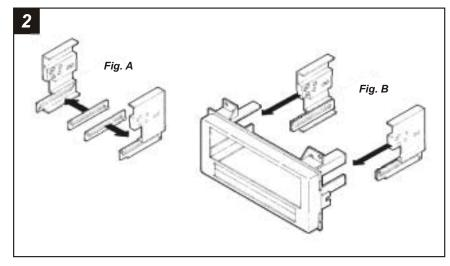
**IF AN EQUALIZER WILL NOT BE INCLUDED:** Skip to step #3. **IF AN EQUALIZER WILL BE INCLUDED:** Snap the **Equalizer Spacers** onto the bottom of the **ISO-DIN Brackets.** (see Fig. A). Slide the Brackets onto the **Radio Housing** legs. (see Fig. B)
