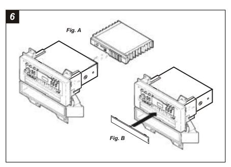
**IF AN EQUALIZER WILL BE INCLUDED:** Slide the aftermarket equalizer into the back of the **Radio Housing.** Using the hardware included with the equalizer, mount the unit to the kit. (see Fig. A)
