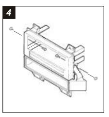
Mount the pocket to the *Radio Housing* with (2) *Carriage Bolts* and (2) *Nuts* supplied.
