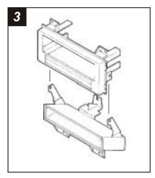
Remove the pocket from the factory head unit and slide the mounting tabs on the pocket over the side tabs on the *Radio Housing*.
