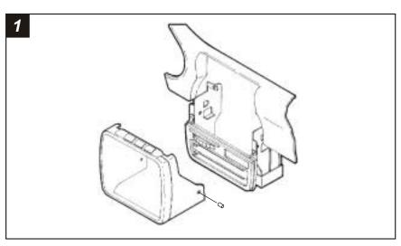
Disconnect the negative battery terminal to prevent an accidental short circuit. Remove (2) pop-clips from the sides of the radio trim bezel. Unclip the radio trim bezel, disconnect the switch wiring and remove the bezel. Remove (2) 7mm hex-head screws securing the top of the factory head unit and disconnect the wiring.
