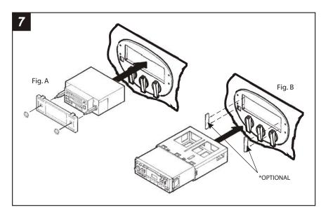
**2-SHAFT HEAD UNITS:** Snap the Faceplate into the Integrated Mounting Kit. Slide the aftermarket head unit into the kit and secure with shaft nuts. (see Fig. A)
