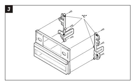
Cut and remove all mounting tabs on **Bracket Set #1** EXCEPT tabs **"C"**. The mounting tabs can be identified by the stamped letter on the back of each tab. Mount the converted Brackets to the back of the assembly with **(6) #8** x ¾" **Hex-head Screws** supplied. Skip to the Installation Instructions for ALL VEHICLES on Page #10.
