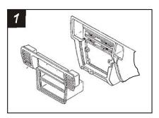
Disconnect the negative battery terminal to prevent an accidental short circuit. Remove (2) screws located under the a/c vents. Remove the climate control knobs. Remove (2) screws above the climate controls. Using a small screwdriver, unclip the top of the dash trim bezel and remove the bezel. Remove (4) Phillips screws securing the factory head unit and disconnect the wiring.
