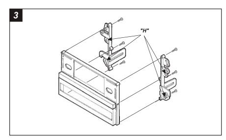
Cut and remove all mounting tabs on **Bracket Set #1** EXCEPT tabs **"H"**. The mounting tabs can be identified by the stamped letter on the back of each tab. Mount the converted Brackets to the back of the assembly with **(6) #8** x ¾" **Hex-head Screws** supplied. Skip to the Installation Instructions for ALL VEHICLES on Page #10.
