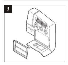
Disconnect the negative battery terminal to prevent an accidental short circuit. Unclip the radio trim bezel and remove. Remove (4) Phillips securing the factory head unit and disconnect the wiring.
