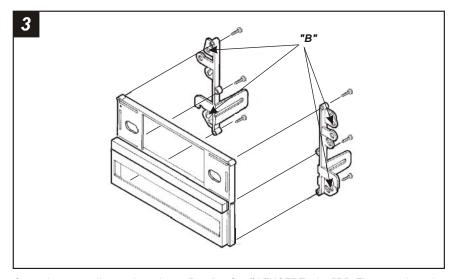
Cut and remove all mounting tabs on **Bracket Set #1** EXCEPT tabs **"B"**. The mounting tabs can be identified by the stamped letter on the back of each tab. Mount the converted Brackets to the back of the assembly with **(6) #8 x ¾" Hex-head Screws** supplied. Skip to the Installation Instructions for ALL VEHICLES on Page #10.
