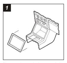
Disconnect the negative battery terminal to prevent an accidental short circuit. Unclip the radio trim bezel and remove. Remove (4) screws securing the factory head unit and disconnect the wiring.
