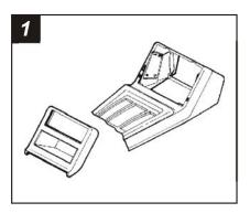
Disconnect the negative battery terminal to prevent an accidental short circuit. Remove the ashtray and (2) screws exposed. Unclip the gear shifter trim bezel and remove (4) screws exposed. Pop off the hazard switch and remove (1) screw exposed. Remove the dummy cap located below the brake lever and (2) screws exposed. Remove the screws securing the factory head unit and disconnect the wiring.
