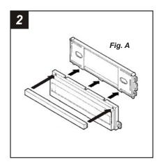
Snap the *Filler Bar* onto the *Equalizer Housing* and slide the assembly onto the bottom of the *Radio Housing*. (see Fig. A). (The factory pocket may be used by omitting this step and mounting the pocket under the Radio Housing during installation).
