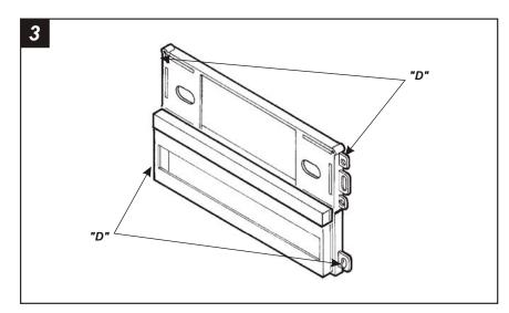
Cut and remove all mounting tabs on the *Radio Housing* EXCEPT tabs "D". The mounting tabs can be identified by the stamped letter on the back of each tab. *Skip to the Installation Instructions for ALL VEHICLES on Page #10.*
