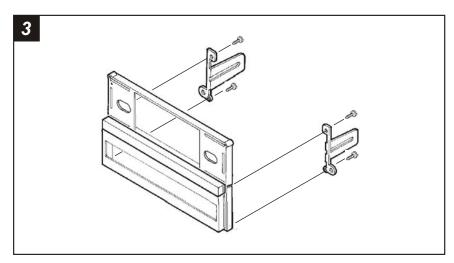
Mount Bracket Set #2 to the back of the Equalizer Housing with (4) #8 x ½" Hex-head Screws supplied. Skip to the Installation Instructions for ALL VEHICLES on Page #10.
