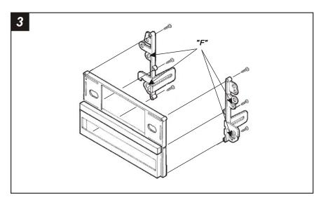
Cut and remove all mounting tabs on **Bracket Set #1** EXCEPT tabs **"F"**. The mounting tabs can be identified by the stamped letter on the back of each tab. Mount the converted Brackets to the back of the assembly with **(6) #8** x ¾**" Hex-head Screws** supplied. Skip to the Installation Instructions for ALL VEHICLES on Page #10.
