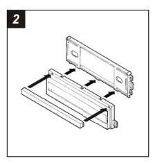
Snap the *Filler Bar* onto the *Equalizer Housing* and slide the assembly onto the bottom of the *Radio Housing*.
