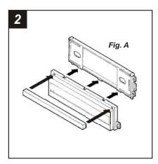
Snap the *Filler Bar* onto the *Equalizer Housing* and slide the assembly onto the bottom of the *Radio Housing*. (see Fig. A). (The factory pocket may be used by omitting this step and mounting the pocket under the Radio Housing during installation).
