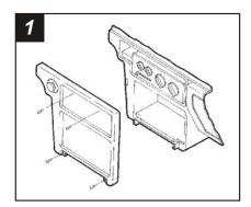
Disconnect the negative battery terminal to prevent an accidental short circuit. Remove the ashtray. Remove (2) Phillips screws above the climate controls. Remove (2) Phillips screws from the bottom edge of the radio trim bezel and remove the bezel. Remove (4) Phillips securing the factory head unit and disconnect the wiring.
