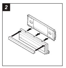
Snap the *Filler Bar* onto the *Equalizer Housing* and slide the assembly onto the bottom of the *Radio Housing*.
