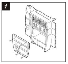
Disconnect the negative battery terminal to prevent an accidental short circuit. Remove (2) screws from the top of the radio trim bezel. Remove the ashtray and (2) screws exposed. Unclip the radio trim bezel and disconnect the cigarette lighter wiring. Remove the screws securing the factory head unit and disconnect the wiring.
