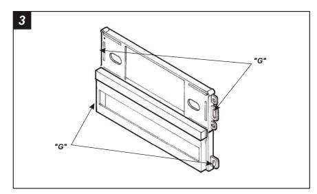
Cut and remove all mounting tabs on the *Radio Housing* EXCEPT tabs "G". The mounting tabs can be identified by the stamped letter on the back of each tab. *Skip to the Installation Instructions for ALL VEHICLES on Page #10.*
