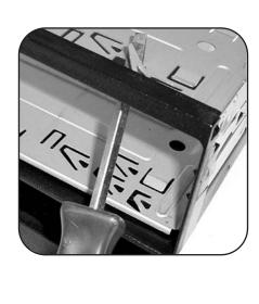
Using the factory hardware, mount the 99-7009 in the location where the factory pocket resided.
