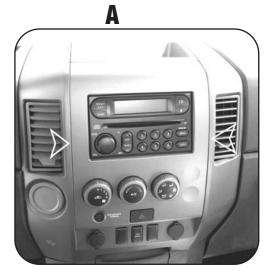
**3** Remove (4) Phillips screws to remove radio. **(Figure B)**
