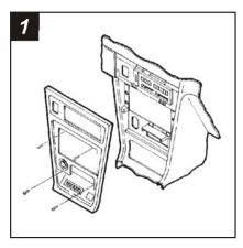
Disconnect the negative battery terminal to prevent an accidental short circuit. Remove (2) Phillips screws above the radio opening. Remove the ashtray and (2) screws exposed in the ashtray cavity. Unclip the top of the dash trim bezel and remove. Remove (4) screws securing the factory head unit and disconnect the wiring.
