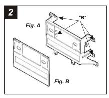
Cut and remove all mounting tabs on the **Radio Housing** EXCEPT tabs **"B"**. The mounting tabs can be identified by the stamped letter on the back of each tab. (see Fig. A). Locate **Faceplate #2**. (see Fig. B). Skip to the Installation Instructions for ALL VEHICLES on Page #2.
