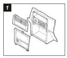
Disconnect the negative battery terminal to prevent an accidental short circuit. Unclip the climate control trim bezel and remove (2) screws exposed. Unclip the gear shifter trim bezel and remove (2) screws exposed. Remove the ashtray and (1) screw exposed. Unclip the radio trim bezel (the factory head unit, pocket and mounting brackets are secured to the bezel). Disconnect the wiring. Remove the screws securing the mounting brackets to the assembly and remove the brackets.
