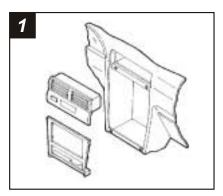
Disconnect the negative battery terminal to prevent an accidental short circuit. Unclip the gear shifter trim bezel and remove (2) screws exposed. Remove (1) screw to the left of the ashtray and unclip the ashtray assembly. Unclip the clock/vent assembly and remove. Remove (4) screws from the top of the mounting bracket assembly. Disconnect the wiring and remove the assembly. Remove the screws securing the mounting brackets to to the assembly and remove the brackets.
