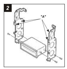
Using a hammer, flatten the protruding screw holes ("A") on the factory mounting brackets. Mount the factory pocket to the brackets with those screws previously removed in step #1. Skip to the Installation Instructions for ALL VEHICLES on Page #2.
