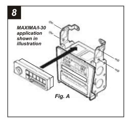
**MAXIMA**, **I-30**: Re-connect the battery terminal and test the unit for proper operation. Mount the climate controls to the factory brackets with (4) screws previously removed in step #1. (see Fig. A). Mount the assembly to the sub-dash with those screws previously removed in step #1.
