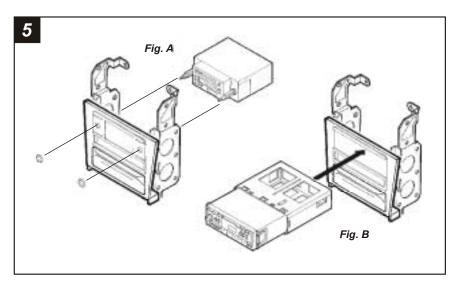
**2-SHAFT HEAD UNITS:** Slide the aftermarket head unit into the mounted **Radio Housing** and secure with shaft nuts. (see Fig. A)
