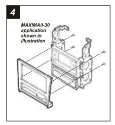
MAXIMA, I-30: Mount the radio trim bezel to the front of the assembly with (4) screws previously removed in step #1. (see Fig. A). 240SX: Mount the radio trim bezel to the front of the assembly with (2) #10 x ¾" Phillips Screws supplied.
