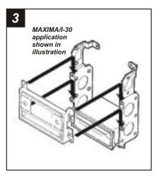
Mount the *Radio Housing* to the factory brackets by sliding the mounting tabs on the Housing down behind the mounting tabs on the brackets.
