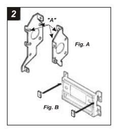
Using a hammer, flatten the protruding screw holes ("A") on the factory mounting brackets. (see Fig. A). Attach the **Spacers** to the upper **Radio Housing** mounting tabs. (see Fig. B). Skip to the Installation Instructions for ALL VEHICLES on Page #2.
