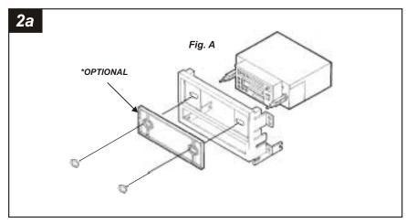
**2-SHAFT HEAD UNITS:** Attach the **Spacer**\* to the **Radio Housing**. Slide the aftermarket head unit into the mounted kit and secure with shaft nuts. (see Fig. A)
