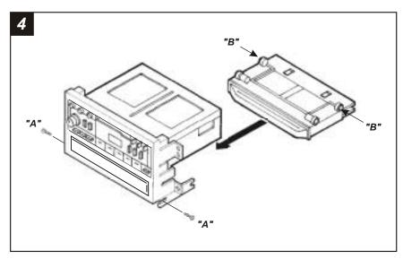
Mount the factory cupholder to the bottom of the *Radio Housing* with (2) Phillips screws previously removed in step #1 ("A") and (2) locating pins ("B").
