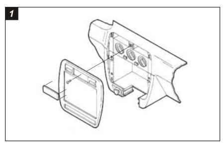
Disconnect the negative battery terminal to prevent an accidental short circuit. Unclip the dummy plate from the center of the switch panel (above the radio opening). Unclip the radio trim bezel and remove. Remove (4) Phillips screws securing the factory head unit and disconnect the wiring. Remove (2) Phillips screws securing the factory cupholder and remove.
