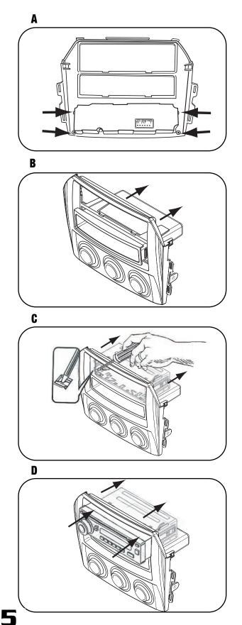
**3** Slide the DIN cage into the Radio Housing and secure by bending the metal locking tabs down. (Figure C)
