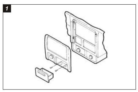
Disconnect the negative battery terminal to prevent an accidental short circuit. Remove the ashtray and (2) Phillips screws exposed in the ashtray cavity. Unclip the radio trim bezel and remove. Remove (4) Phillips screws securing the factory head unit and disconnect the wiring.
