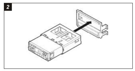
**DIN HEAD UNITS:** Slide the DIN cage into the **Radio Housing** and secure by bending the metal locking tabs down. Slide the aftermarket head unit into the cage until secure. (For a 2-shaft head unit installation, order Metra's **87-09-9902** and snap it into the Radio Housing).
