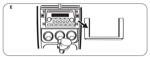
**NOTE:** As an option, the center panel (the smaller piece around radio) is all that needs to be removed, but it is very prone to damage, so full panel removal is recommended. (Figure C)
