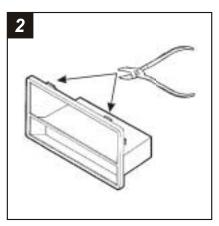
Cut and remove the *TOP* clips from the *Radio Housing*.
