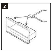
Cut and remove the TOP clips from the  $\it Radio\,Housing.$
