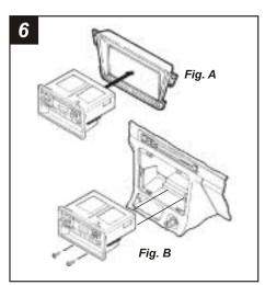
ACCORD 1990-93, INTEGRA, ODYSSEY, OASIS: Re-connect the battery terminal and test the unit for proper operation. Snap the head unit/kit assembly into the sub-dash.
