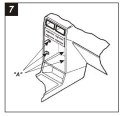
Locate the (4) mounting positions in the sub-dash ("A").
