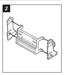
Insert the mounting tabs on the *Radio Housing* into the slots in the *Brackets*.
