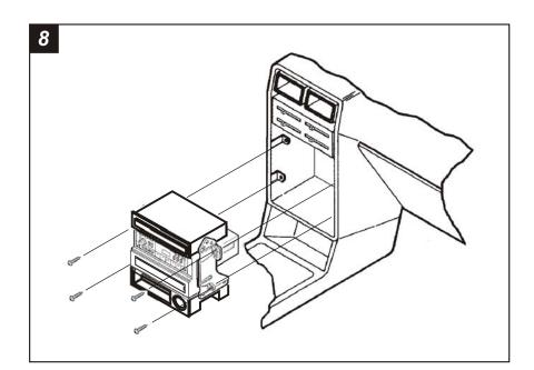
Re-connect the battery terminal and test the unit for proper operation. Mount the head unit/kit assembly to the sub-dash with (4) screws previously removed in step #1.
