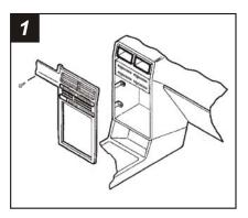
Disconnect the negative battery terminal to prevent an accidental short circuit. Remove (1) Phillips screw located above the ignition switch. Remove the climate control knobs. Unclip the dash trim bezel and remove. Remove (4) Phillips screws securing the factory head unit assembly and disconnect the wiring. Remove (2) screws securing the factory cupholder to the assembly and remove. Remove (4) screws securing the ashtray/cigarette lighter to the assembly and remove.
