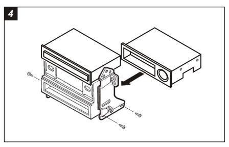
Place the factory ashtray/cigarette lighter below the *Radio Housing* and secure to the *Brackets* with (4) screws previously removed in step #1.
