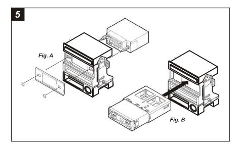
**2-SHAFT HEAD UNITS:** Attach the **Faceplate** to the **Radio Housing.** Slide the aftermarket head unit into the kit and secure with shaft nuts. (see Fig. A)
