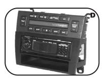
4 Slide the head unit/bracket assembly into the radio opening until the side clips engage.
