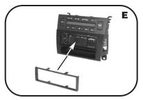
5 Snap the ISO Trimplate over the head unit.
