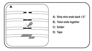
Locate the factory wiring harness in the dash. Metra recommends using the proper mating adapter and making connections as shown. (Isolate and individually tape off the ends of any unused wires to prevent electrical short circuit.)
