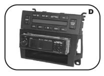
1 Secure the Mounting Brackets to the housing/pocket assembly by snapping securing in place.
