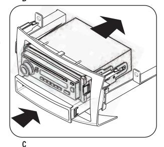
4 Snap the Trim plate onto the front of the Radio Housing assembly. (Figure C)
