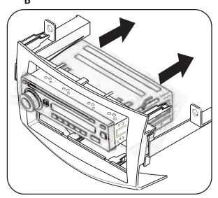
3 Snap the pocket into the radio housing. (Figure C)
