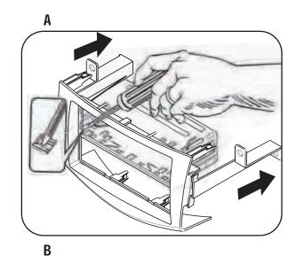
2 Slide the aftermarket radio into the cage until it snaps into place. (Figure B)
