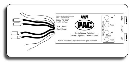
5. Gray/Blk trigger wire: Connecting this wire to chassis ground will switch the AS21 to Auxiliary 2.
