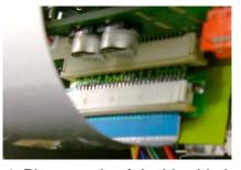
4: Place a strip of double sided tape on the metal. This is to insulate against shorts Plug interface connector in then, reconnect the silver ribbon cable.
