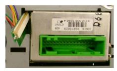
2: Slide the connector into the radio chassis
