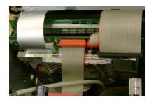
3:Carefully separate the 2 sections. Locate the silver ribbon cable and gently disconnect.
