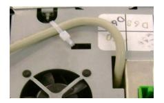
5: Secure the cable coming out of the back as pictured above and reassemble chassis.
