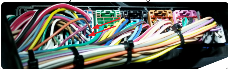
Picture of the BCM which is located under the driver side of the dash just above the steering column
