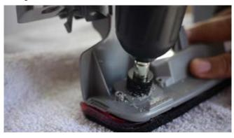
**Step 2**. Continue drilling through the back and into the front side of that brake light. This will allow you a guide hole when you begin drilling on the front side.
