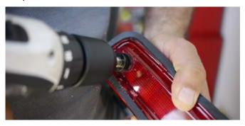
**Step 4**. Clean and clear the hole for the camera to be inserted.
