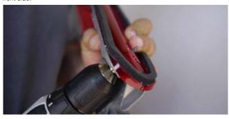
**Step 3**. Turn over the brake light and continue clearing the hole on the front side of the brake light. Be very careful when drilling, take your time and cleanly drill.
