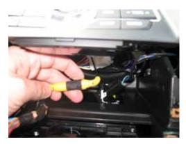
7. Plug the SONATA-CAM module into the 18 pin molex connector and secure the module in the dash with velcro or double sided tape (not provided). Reinstall the radio in the dash.
