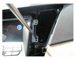
5. Disconnect all wiring from the radio and set it aside in a safe place.
