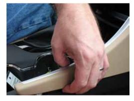
2. Once removed, this will reveal a screw on either side just below the HVAC trim bezel. Remove these two screws
