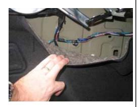
10. Install your rear view camera (not provided) and run the video RCA from the camera and the power wires into the trunk lid. Attach the video RCA from the SONATA-CAM module to the video RCA from the rear view camera. Attach the ground wire from the rear view camera to the BLACK wire at the reverse light three pin plug. Attach BOTH the camera power wire and the power wire from the SONATA-CAM to the BLUE wire at the reverse light in the three pin plug.
