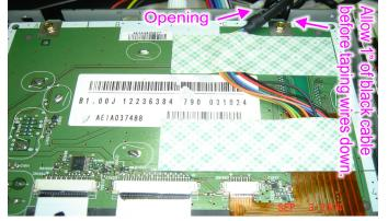
Make sure that the ribbon contacts are straight in the connector after it is taped down.
