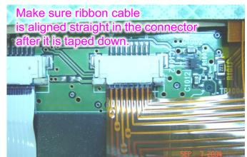
Replace the cover to the radio. Let the ribbon cable Step 6 fold over by itself when replacing cover. **Do not press** the ribbon cable down by hand. Doing so may put a crease into
