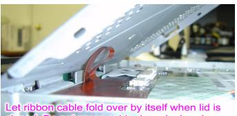
not press cable down by hand. o may damage the circuit traces.2004
