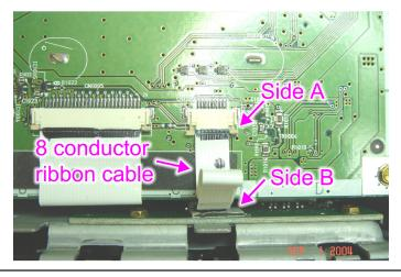
Insert the VCI-GM1/AV ribbon cable into the secondary circuit board connector (nickle plated contacts needs to face away from circuit board). Apply ribbon cable to the double stick tape to hold it in place.
