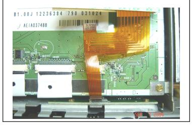
Insert second set of contacts into the main connector (contacts need to be facing upwards).
